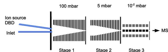
**Figure 2** A schematic drawing of the CIMS transfer stage.
