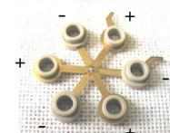
**Figure 3** The two smallest electrodes of the ion funnel with the PEEK spacers.
