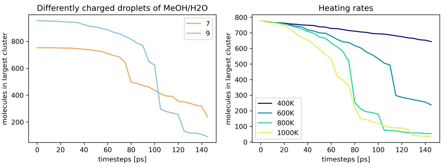
Fig. 1: Fragmentation of droplets in dependency of charge (left) and final temperature (right)
