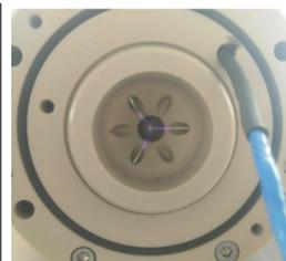
Figure 4: Picture of the corona discharge with three needles in Y-Position.
